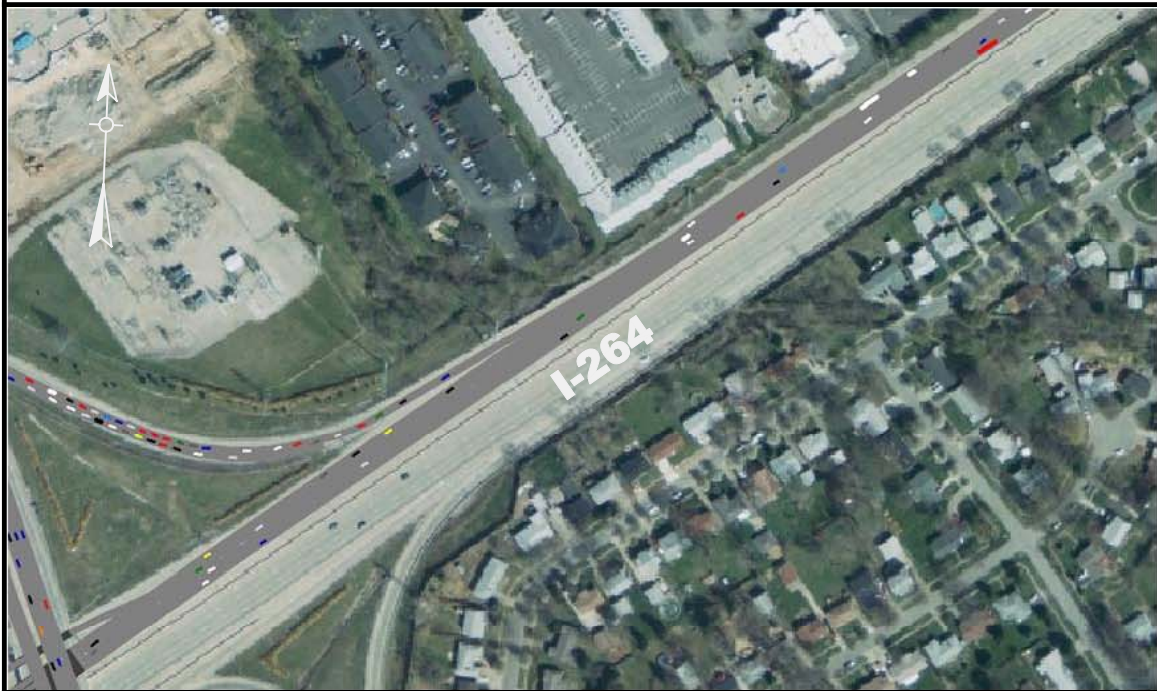
2010 PM - I-264 from I-64 to Breckenridge Lane: Similarly, longer queues on exit ramp when compared to the 2005 PM scenario with heavier mainline volumes.
